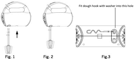
3. To eject the mixing accessories, hold the mixing heads with one hand and press the eject button firmly with the other.
